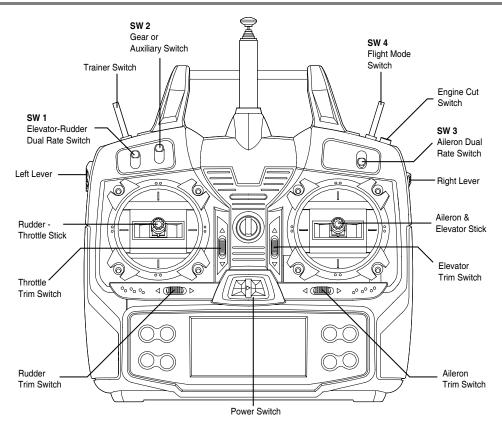
This figure shows the assignments for a **Mode 2** system as supplied by the factory in North America.
