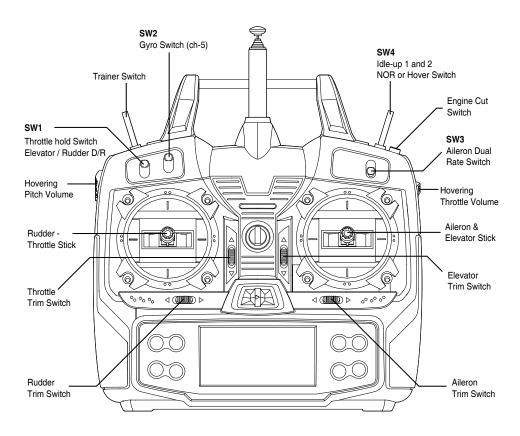
This figure shows the assignments for a **Mode 2** system as supplied by the factory. Note that some of the functions will not operate until activated in the mixing menus.
