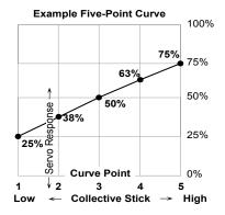
You can get a linear response by making the five settings line up as shown above. But if you want another shape, you're free to do it. You can "flatten out" or "soften" the curve around hover as shown here. This is handy for making the control less sensitive around hover.
